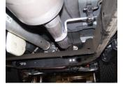
stock nuts/bolts. Insert welded hanger into rubber grommet. DO NOT TIGHTEN. **4.** Install muffler #B onto head pipe #A 1½"-2". Muffler outlets
